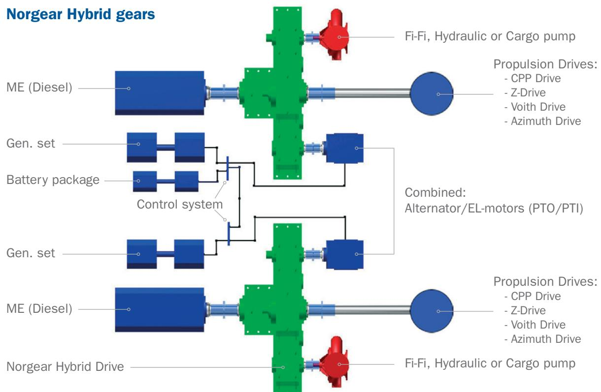
The Norgear Hybrid gears are available with and without auxiliary drives for Fi-Fi, Hydraulic and cargo pump drives. Built in multidisc hydraulic clutches with soft engagement are standard.
