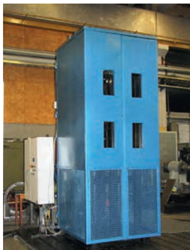
This testing chamber enables full load testing of Anode Jacks in high ambient temperature upto 150 °C.
