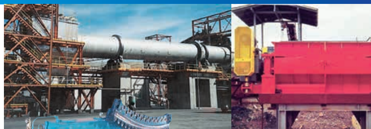
Kumera Drives supplies complete functional packages for rotary drum drives including gear units, pinion wheel, girth gears and assembly base.
