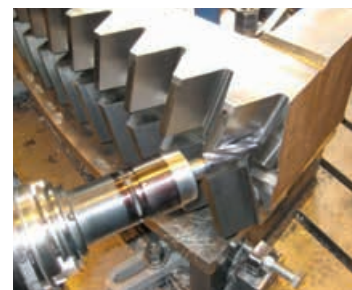
Accurate machining of tooth profile
